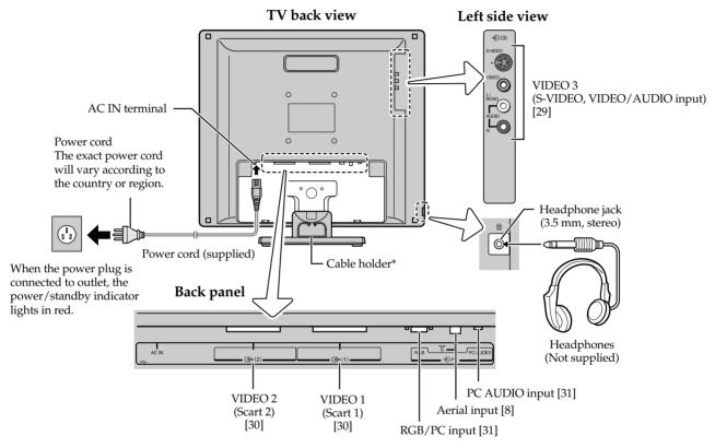
You can use the cable holder to hold the aerial and audio/video cables. Never use the cable holder to carry the TV when moving it.
